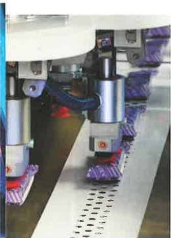
The vacuum gripper turns product 90° and transfers for further processing.
