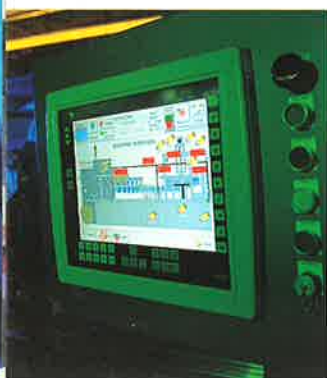
Touch screen control panel incorporates diagnostics, maintenance, and trouble shooting data in an operator-friendly format.
