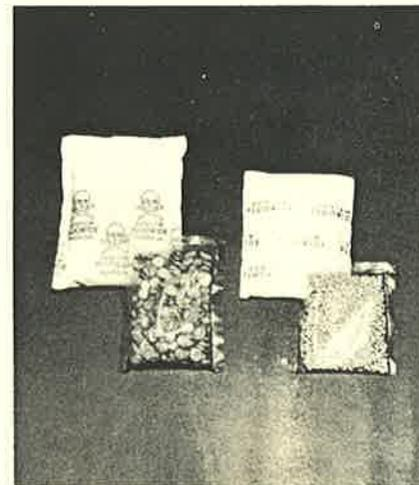
Gilliam-Packaged sodium fluoride and aluminum shot used as fluxing agents for use in steel making process
